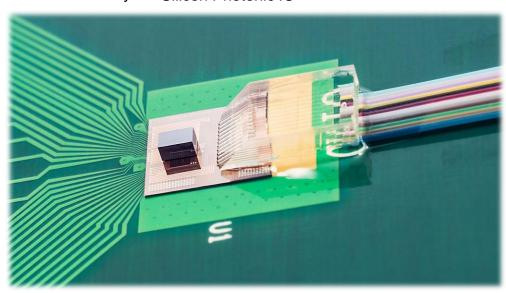
TSV-enabled Hybrid FinFET CMOS – Silicon Photonics Technology for High Density Optical I/O
